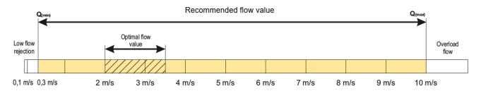
Figure 8. Recommended flow values for the PEM-500 flowmeter.
