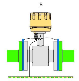
Figure 6. Example of functional earthing connection for metallic (A) piping and for insulated piping using earthing rings (B).
