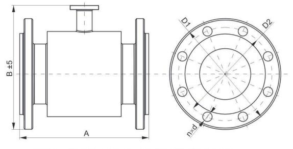
DN 10 - DN 150 A ± 5 mm, DN 200, DN 250 A ± 10 mm
