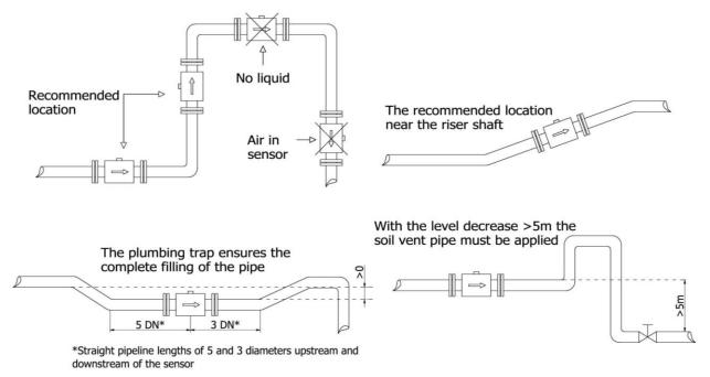
Figure 4. Recommended installation of the sensor.
