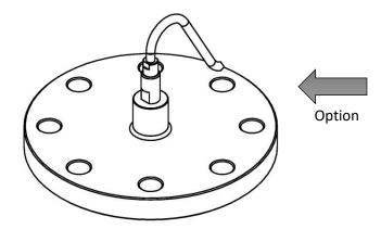
Figure 80. Types of flange separators S-P.
