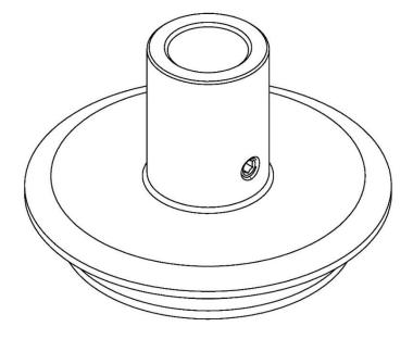
Figure 128. S-Varivent DN50 separator - view in isometry.
