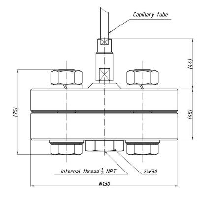
Figure 95. S-Comp10MPa separator - overall dimensions.
