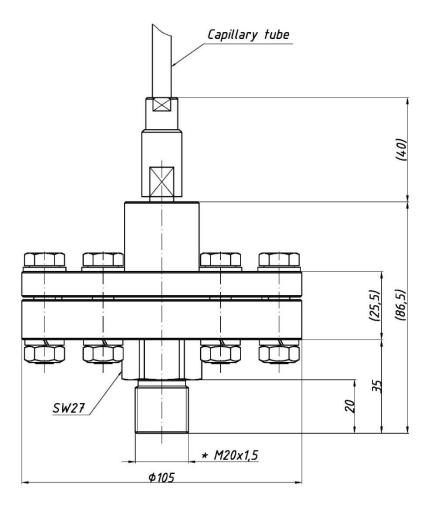
Figure 89. S-CompK separator - overall dimensions.
