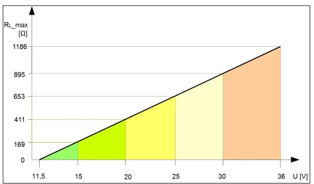
Figure 28. The maximum load resistance  $R_{L_{MAX}}[\Omega]$  in the supply line of transmitter in Exi/Exd version without backlight depending on the power supply voltage U [V].
