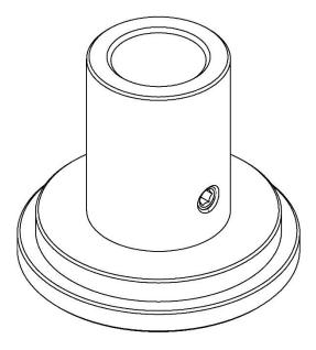
Figure 110. S-SMS separator. View in isometry.
