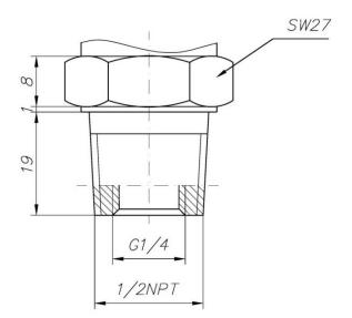
Figure 44. Type  $\frac{1}{2}$  NPT connection (ext.  $\frac{1}{2}$  NPT, inner G  $\frac{1}{4}$ ").
