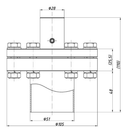
Figure 91. S-Comp ø51 separator - overall dimensions.
