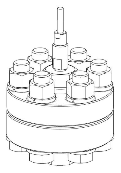
Figure 98. S-Comp60MPa separator - view in isometry.
