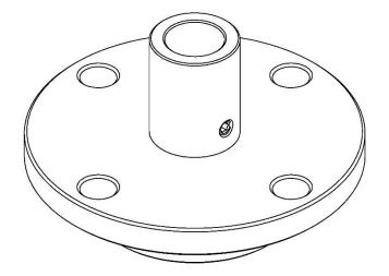
Figure 124. S-DRD 65 separator - view in isometry.
