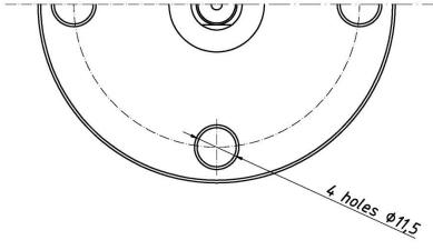
Figure 127. S-K DRD 65 (distance separator with capillary in axis) - overall dimensions.
