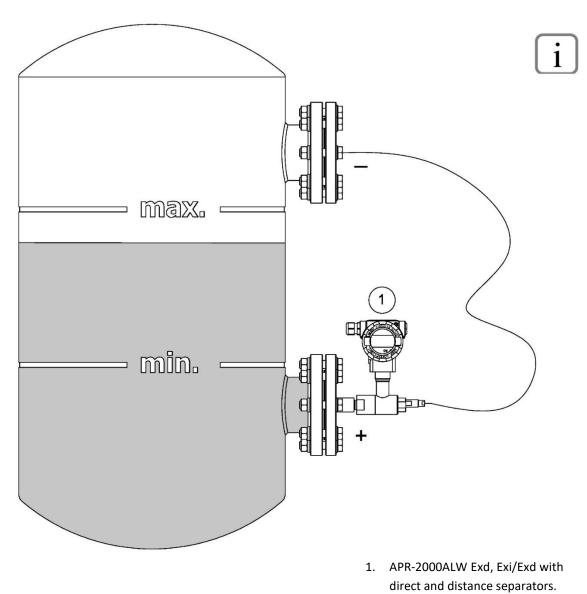
Figure 11. Liquid level measurement in closed tanks using APR-2000ALW Exd, Exi/Exd with direct and distance separators.
