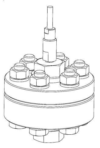
Figure 96. S-Comp25MPa separator - view in isometry.
