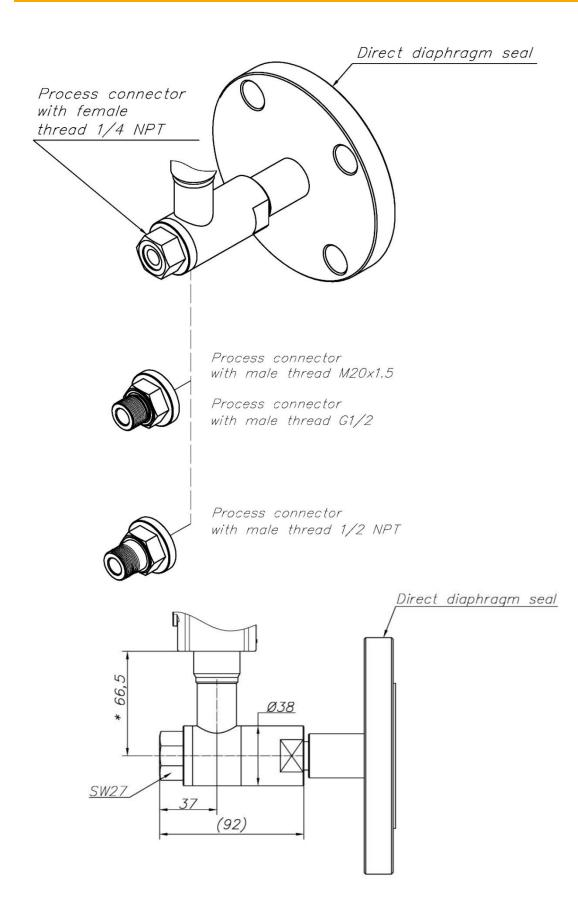
Figure 75. Direct separator and possible process connections.
