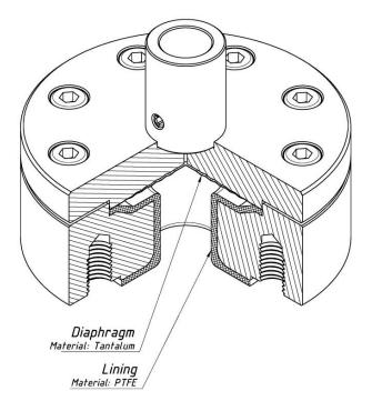
Figure 104. S-CompCh DN25 separator in half section view.
