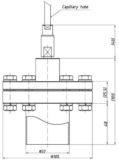
Figure 93. S-CompK ø51 - overall dimensions.
