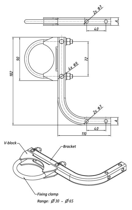
A = 16 Bracket AL (galvanized) A = 15 Bracket AL (stainless steel)
