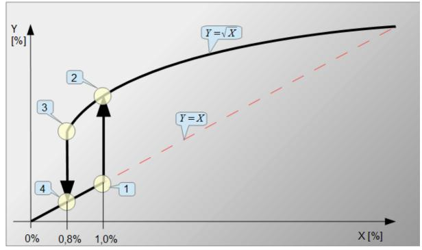
Figure 25. Manufacturer's root characteristics 2 with adjustable dead band and hysteresis 0.2%.
