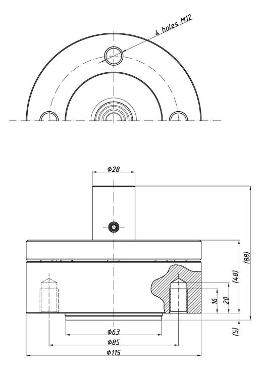
Figure 105. Separator S-CompCh DN25 - overall dimensions.
