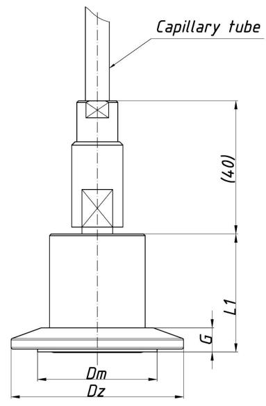
Figure 117. S-K Clamp separator - overall dimensions.
