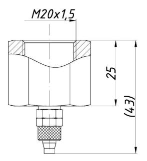
Figure 58. Elastic tube ø6x1.
