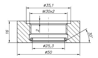
Figure 47. Type CM30x2 connection (M30x2) with socket and ring.
