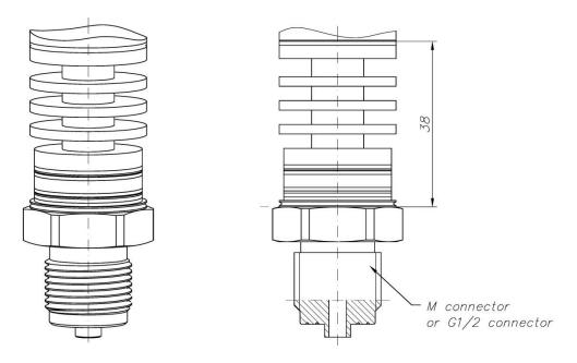
Figure 51. Radiator with M20x1,5 or G ½ stub.
