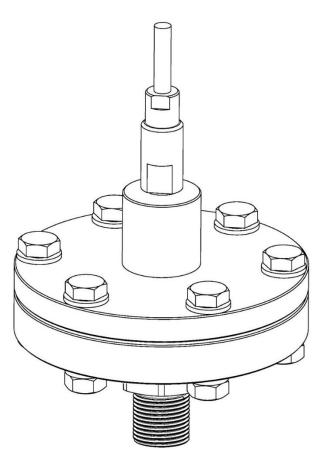
Figure 88. S-CompK distance separator with capillary in axis.
