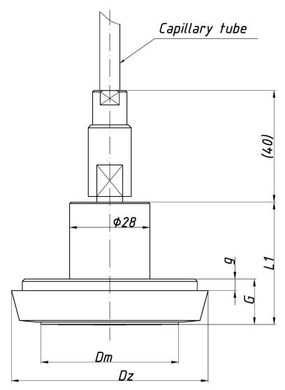
Figure 109. S-K DIN separator with capillary in axis - overall dimensions.
