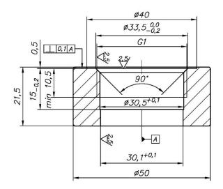
Figure 48. Type CG1 connection (G1") with socket.
