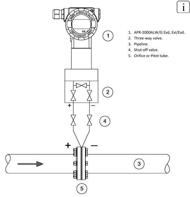
Figure 2. Gas flow rate measurement system using APR-2000ALW/G Exd, Exi/Exd.
