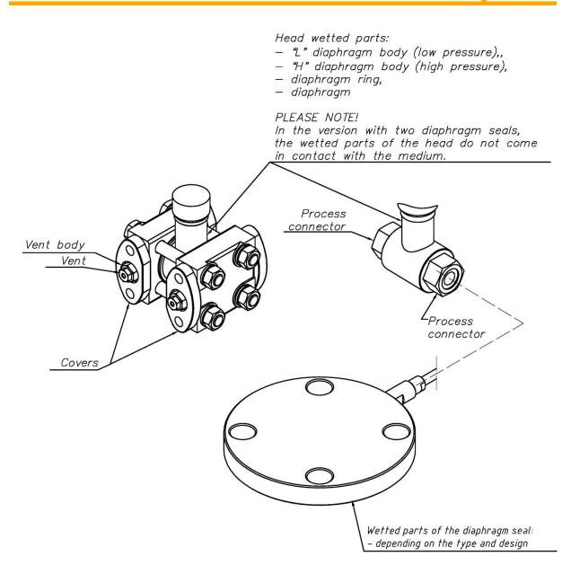
Figure 73. Specification of materials coming into contact with the process for APR-2000ALW Exd, Exi/Exd.
