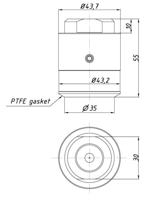
Figure 118. S-Poziom 25 separator - overall dimensions.
