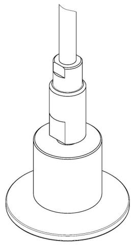
Figure 116. S-K Clamp separator (distance separator with capillary in axis).
