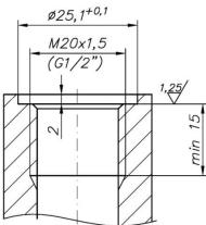
Figure 46. Type GP connection (G  $\frac{1}{2}$ , Ø12) with socket.
