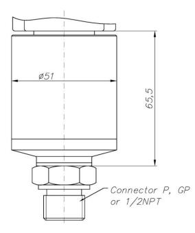
Figure 64. Process connection HS.
