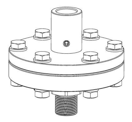
Figure 86. S-Comp separator - view in isometry.
