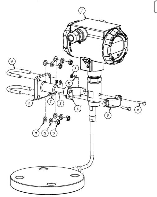
Figure 37. Assembly and mounting of the variant with distance separator.
