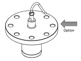
Figure 82. Types of flanged tubular separators S-T.
