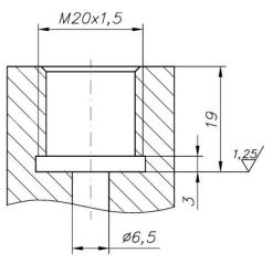
Figure 42. Type M connection (M20x1.5, Ø4) with socket.
