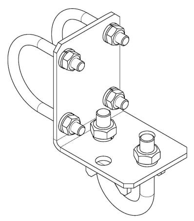
Figure 69. Mounting bracket Ø25 - view in isometry.
