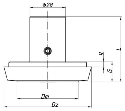
Figure 107. S-DIN - overall dimensions.
