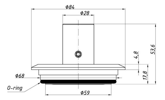
Figure 129. S-Varivent DN50 separator - overall dimensions.
