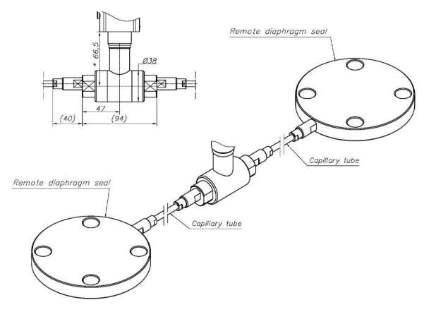
Figure 77. Example of connection using two distance separators.
