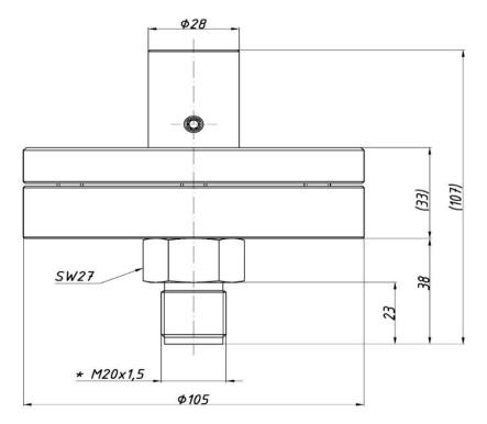
Figure 102. S-CompCh - overall dimensions.
