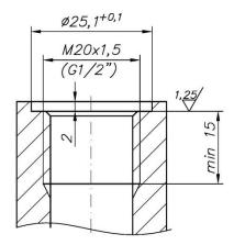
Figure 43. Type P connection (M20x1.5, Ø12) with socket.
