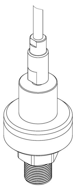
Figure 134. S-MazutK distance separator with capillary in axis. View in isometry.
