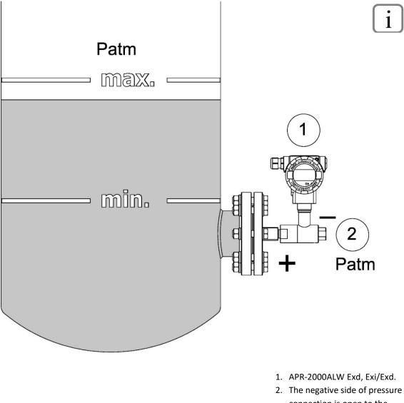
The negative side of pressure connection is open to the atmosphere.
