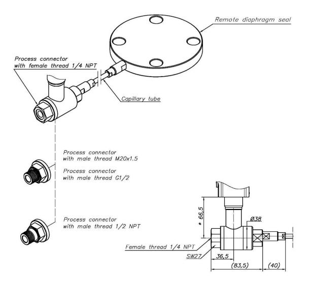
Figure 76. Distance separator and possible connections.
