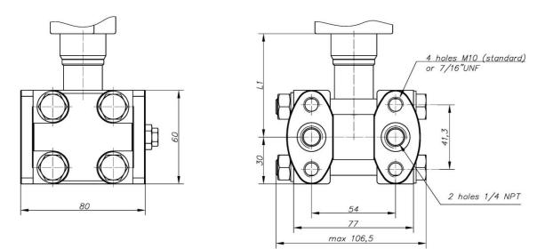
Figure 60. Overall dimensions of type C connection.
