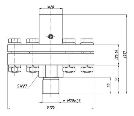
Figure 87. S-Comp separator - overall dimensions.
