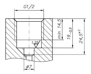
Figure 45. Type G  $\frac{1}{2}$ " connection (G  $\frac{1}{2}$ ", Ø4) with socket.
