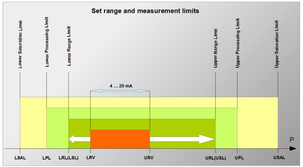
Figure 22. Set range and measurement limits.
