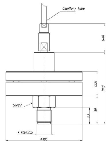
Figure 103. S-CompChK with capillary in axis - overall dimensions.
