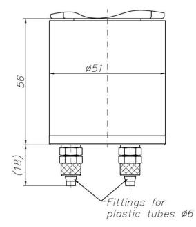
Figure 62. Process connection PCV type.
