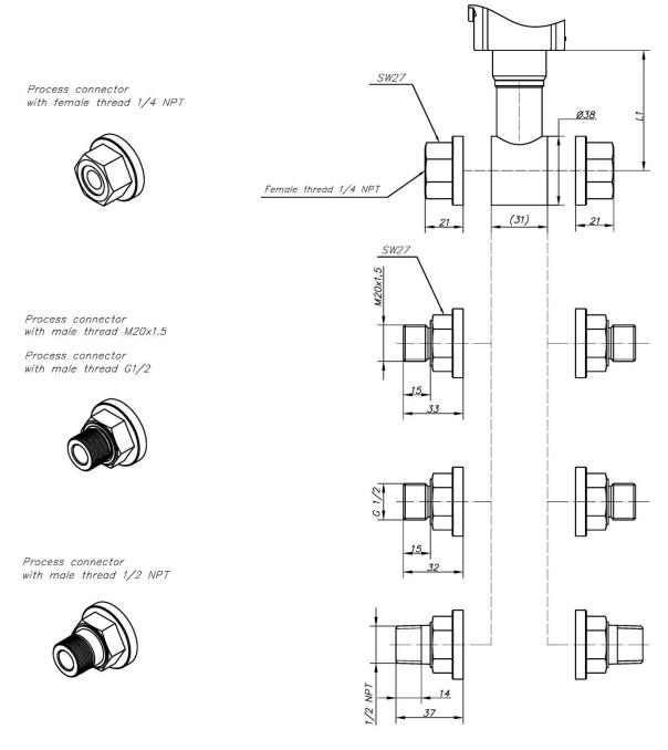
Figure 59. Type P connection for APR-2000ALW Exd, Exi/Exd.
