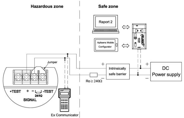
Figure 30. Electrical connection 4...20 mA of HART to transmitter in Exi version
