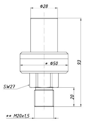
Figure 133. S-Mazut separator - overall dimensions.
