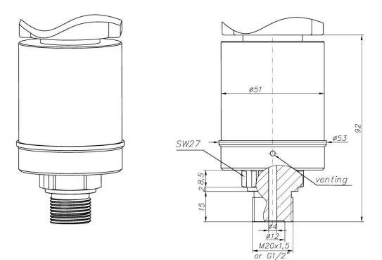
Figure 63. Process connection P or GP for low pressure gases measurement.
