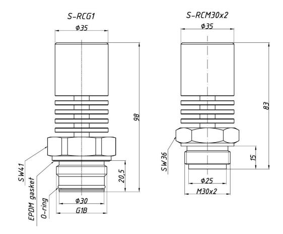
Figure 138. S-RCG1 and S-RCM30x2 separators - overall dimensions.
