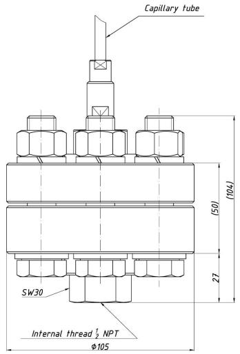
Figure 99. S-Comp60MPa separator - overall dimensions.
