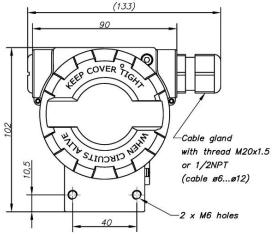
Figure 40. Overall dimensions of APC(R)-2000ALW Exd, Exi/Exd.
