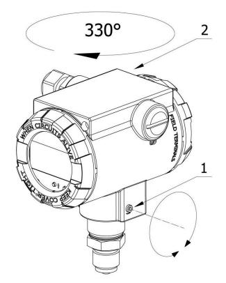
Figure 38. Rotation of APC(R)-2000ALW Exd, Exi/Exd transmitter housing.
