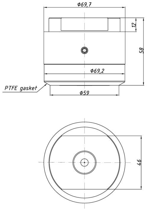
Figure 121. S-Poziom 50 separator - overall dimensions.
