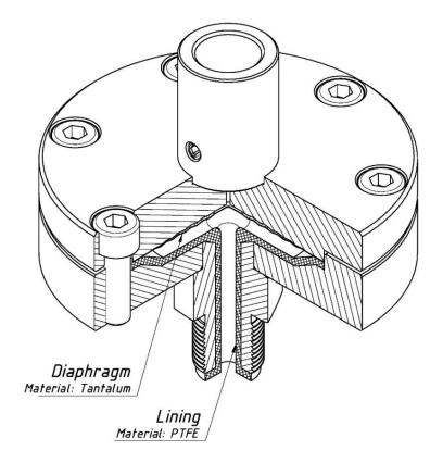
Figure 101. S-CompCh - view of half section.
