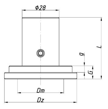
Figure 111. Overall dimensions of separator S-SMS.
