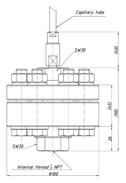
Figure 97. S-Comp25MPa separator - overall dimensions.
