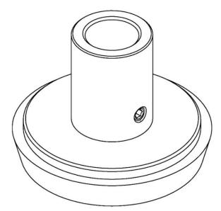
Figure 106. S-DIN separator. View in isometry.
