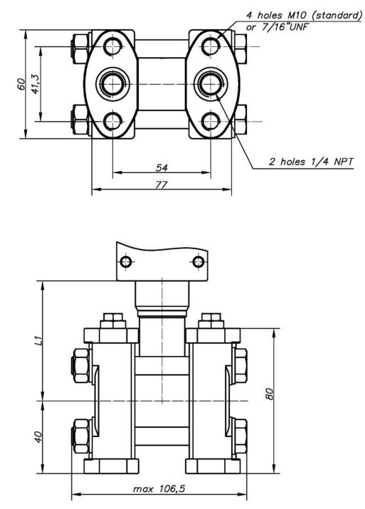
Figure 61. Overall dimensions of CR type connection.
