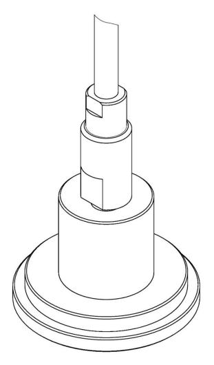
Figure 112. S-K SMS separator with capillary in axis. View in isometry.
