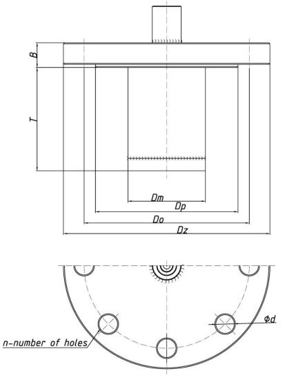
Figure 81. Flanged seals with extended diaphragm S-T.
