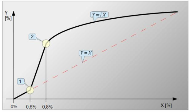
Figure 24. The manufacturer's root characteristics 1 with fixed points of the characteristic change at points 0.6% and 0.8%.
