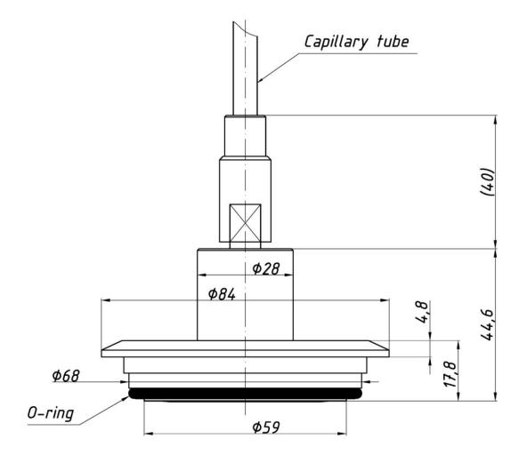
Figure 131. S-K Varivent DN50 (distance separator with capillary in axis) - overall dimensions.
