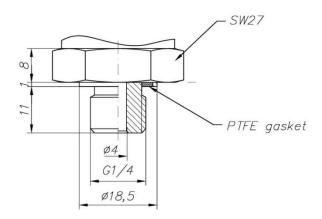
Figure 49. Type G  $\frac{1}{4}$  connection (G  $\frac{1}{4}$ ",  $\frac{0}{4}$ ).
