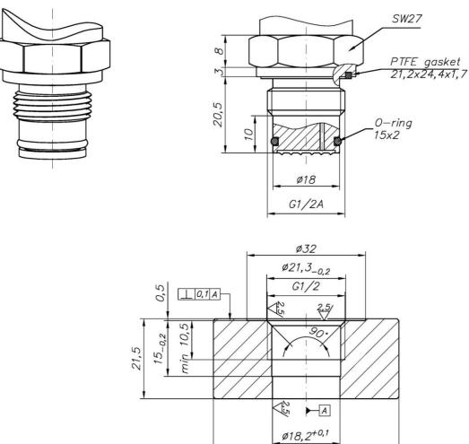
Figure 50. Type CG $\frac{1}{2}$  connection (G  $\frac{1}{2}$ ") with socket.
