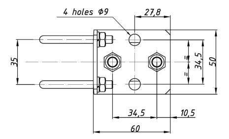
Figure 70. Overall dimensions of the mounting bracket ø25.
